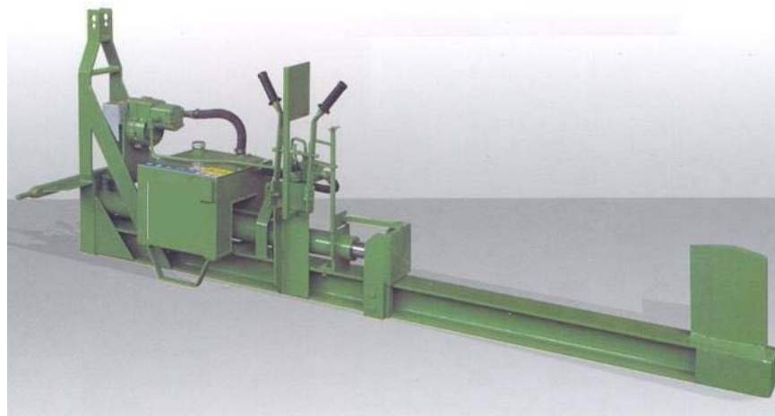
Figure 2. Example of an horizontal log splitters where the activation of two-hand controls used to start the splitting process could be made with parts of the body (hand, arm, etc.)
